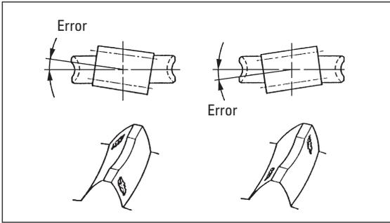
Fig. 19-6 Poor Contact Due to Shaft Angle Error
