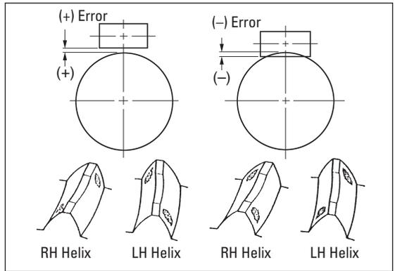
Fig. 19-7 Poor Contact Due to Center Distance Error
