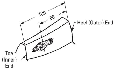
**Fig. 19-1 The Contact Trace on Central Front End**
