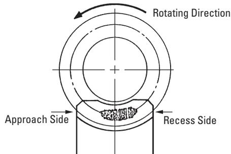
**Fig. 19-5 Ideal Surface Contact of Worm Gear**
