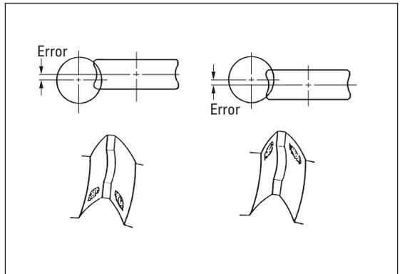
Fig. 19-8 Poor Contact Due to Mounting Distance Error
