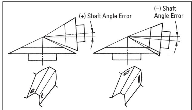
**Fig. 19-3 Poor Contact Due to Shaft Angle Error**
